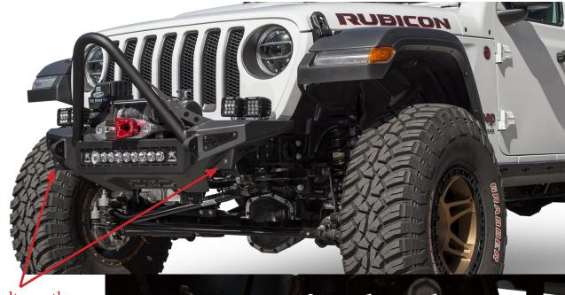
Use 1/2" Bolts on these holes. Install 3/8" Bolts from the back side of the frame horn for the rest of the bolts.
