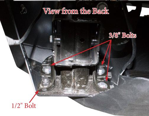
12. Adjust the bumper so that it is straight in relation to the vehicle's grille. Then, torque the 3/8" mounting bolts to 20 foot pounds and torque the 1/2" mounting bolts to 70 foot pounds.
