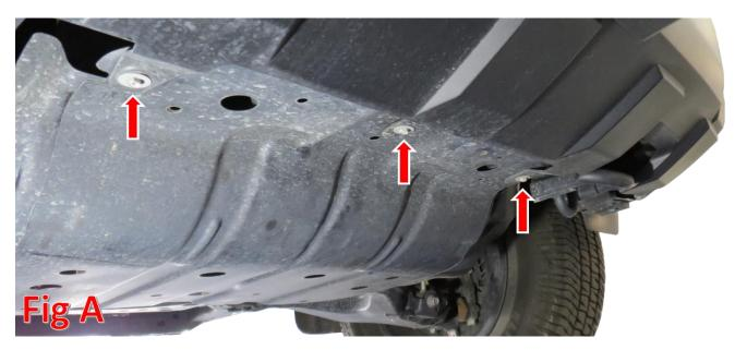
3. Using a 12mm Socket, remove the 5 skid plate bolts, then remove the skid plate. Save these bolts for reuse. (Fig B)
