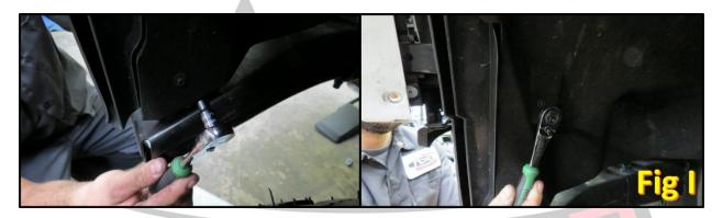
12. Remove the 3 bolts referenced in Fig J on the air dam that sits behind the headlight bezel.
