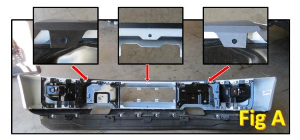
3. Carefully remove the front plastic piece from the bumper. There are no tools required for this, it can be pulled off by hand.
