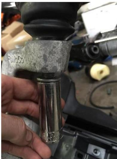
6. Remove lower ball joint nut using a 21mm socket.
