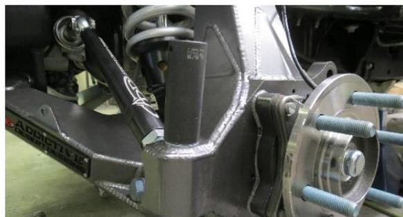
13. Zip tie brake lines, abs line, and vacuum lines to the spindle using the slots in the spindle.
