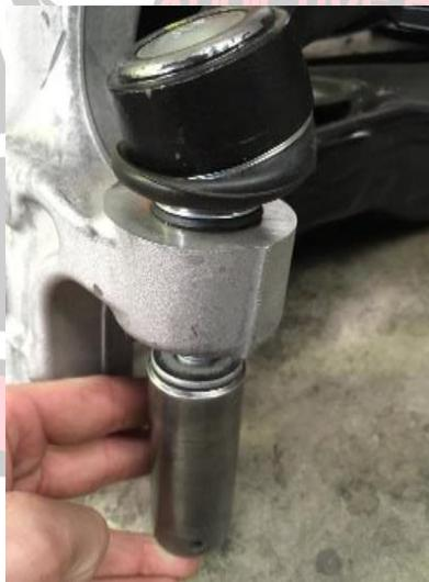
5. Remove upper ball joint nut using a 18mm socket.
