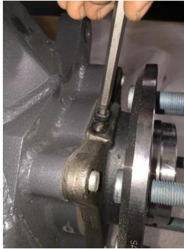
4. Remove tie rod end nut using a 21mm socket.
