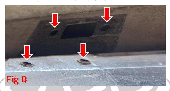
2. Hold your new ADD Side Steps in place and loosely install the provided 5/16" Bolts (x8) and Washers (x8). (Fig B)
