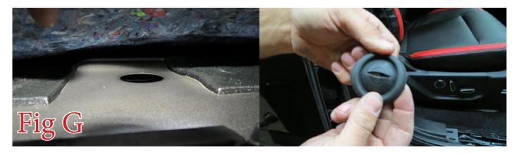
10. Send the red and black wires down the driver side of the frame rail underneath the truck. Then, pass them into the cab through the newly cut grommet. You may need to extend the wires for them to reach.
