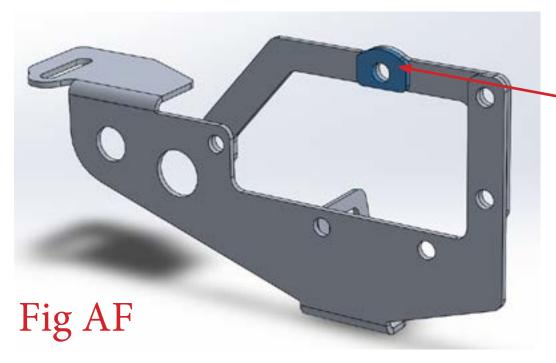
Make sure to sandwich this plate between the module and the bracket.
