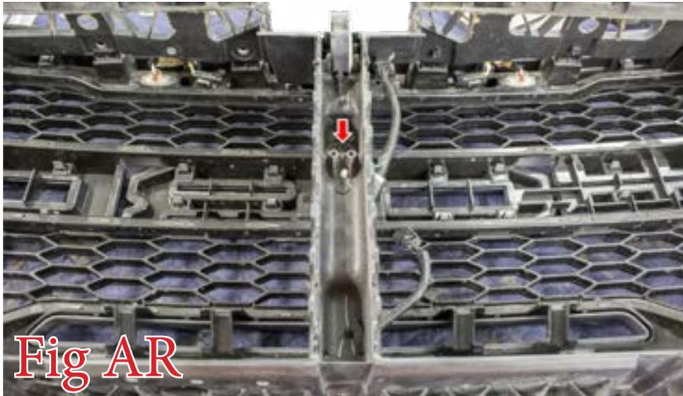
46. Remove the shutter motor from your grille. The tab on the back side of the motor pulls out from the side. Then, the motor will be free to remove. Save this motor. (Fig AS)
