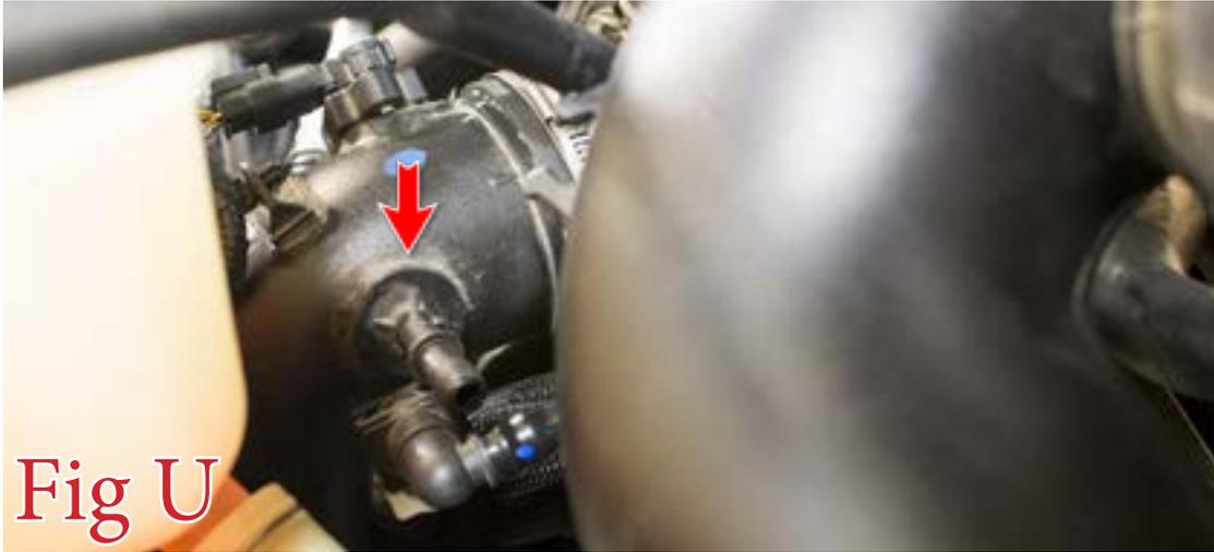
22. Unplug the MAP sensor connector on the tube coming off your throttle body. Also, remove the plastic clip holding the sensor harness to this same pipe. (Fig V)
