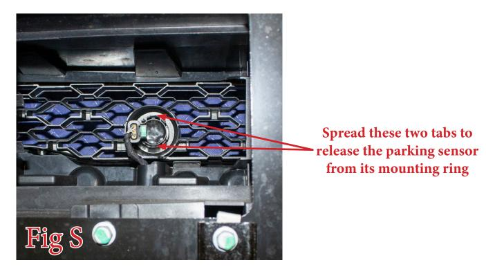
20. Remove the inner four sensor rings. Do this by pressing in the tabs along the base of the sensor rings and pushing the rings out the front side of the bumper. **Make sure to keep track of the position/orientation they come off your OEM bumper so you can reinstall them in the same position/orientation on your new bumper.** (Fig T) **You do not need to remove the outer two sensor bezels.**
