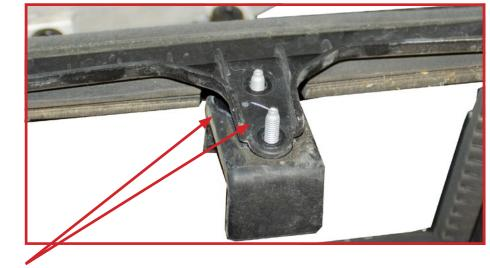
Separate the rubber clamp from bracket
