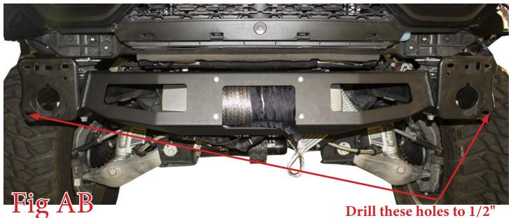
30. Set the bumper in place on the vehicle. Use the supplied 3/8" Hex Head Bolts (2 per side) and 3/8" Washers (2 per side) in the upper mounting holes. In the holes that were drilled out in Step 25, use the supplied Black 1/2" Bolts (1 per side), Black 1/2" Washers (1 per side), and Black 1/2" Lock Nuts (1 per side). Leave these bolts loose for now. (Fig AC)
