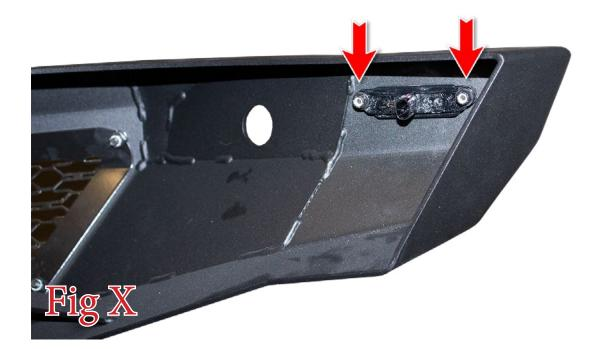
25. Install your light bar and cube lights now. For the light bar, use the supplied light mount kit. The installation instructions for that kit can be found here:
