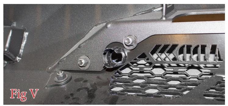
23. On the two outer sensor locations install the sensors in the provided bezels with the skinny side facing up. You will notice that one side will be oriented the same as factory and the driver side will be 180 degrees opposite. \*\*Also note that the sensor plug needs to be 90 degrees to the ground\*\* If your sensor bezel is loose in the bumper and can easily be rotated we recommend applying a small dab of silicone or epoxy to the back side to prevent them from rotating.
