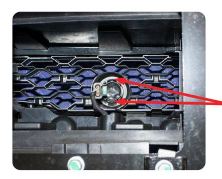
Spread these two tabs to release the parking sensor from its mounting ring
