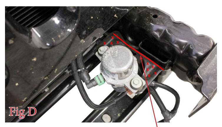
Remove/Relocate this pump, then cut the mount off at the red line.
