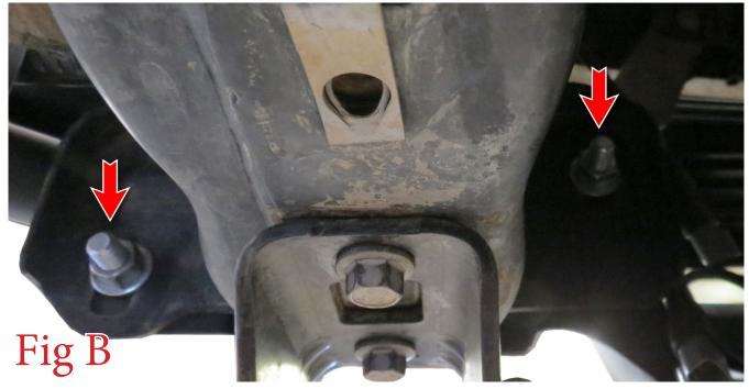
4. Remove the OEM bumper from the vehicle.
