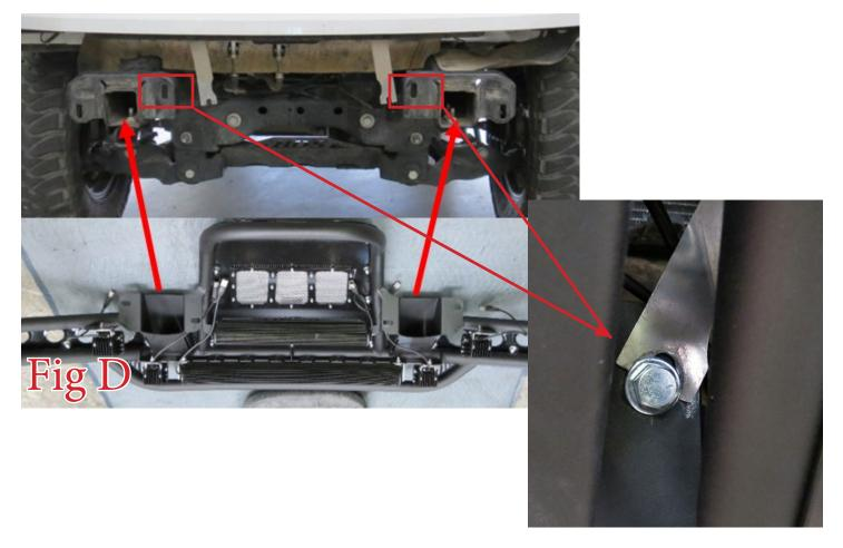
8. Align your bumper so it is centered left to right and also straight in relation to the valance/grille/headlights. Then, tighten the outer mounting bolts to 70 foot pounds.
