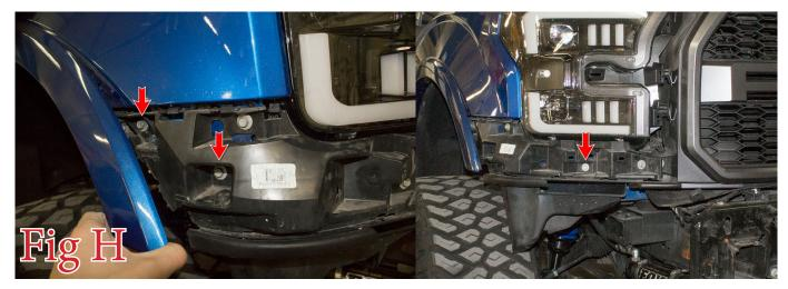
10. Push the headlight bezel back onto the vehicle and reinstall the plastic clip that was removed in Step 5. Then, push the fender flare back into place and reinstall the 7mm bolts you removed in Step 6.
