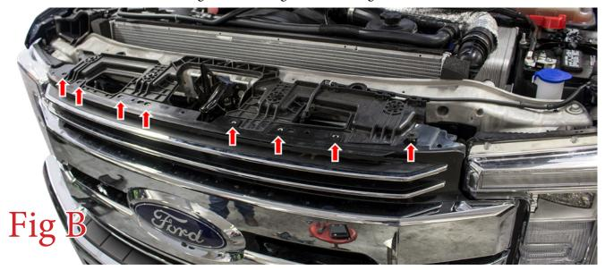
3. Pull the grille off. As you are pulling the grille off, make sure to unplug the front camera and water line (on the back side of the grille). (Fig C)
