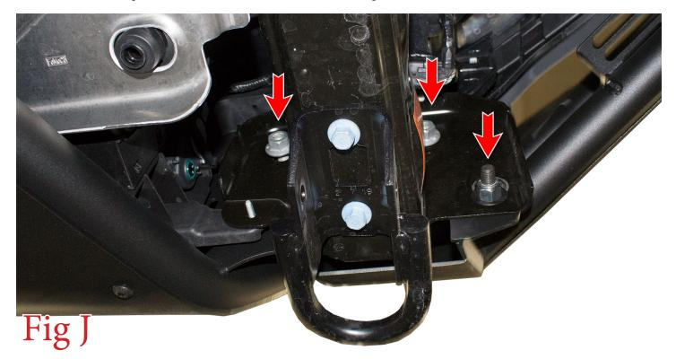
16. Center the bumper left to right and align it so it is straight in relation to the grille/valance. Then, torque the supplied mounting bolts to 70 foot pounds and the OEM bolts to OEM torque spec.
