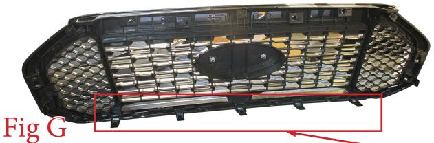
Release this series of clips to remove the grille from the vehicle
