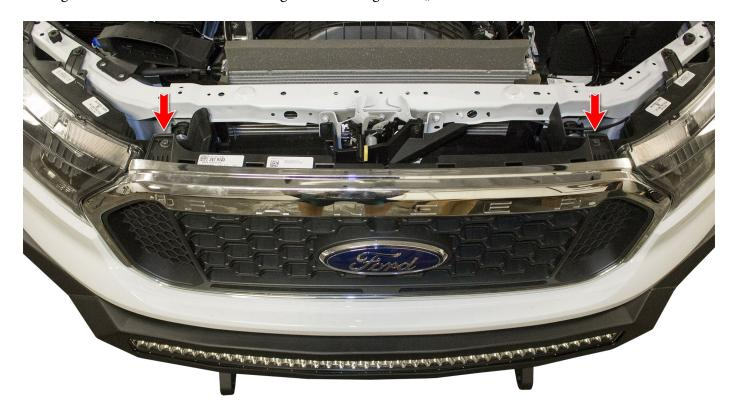
7. Using a T-25 Torx Socket, remove the four mounting bolts for the plastic tray that sits behind the grille. With the four bolts removed, remove that piece.
