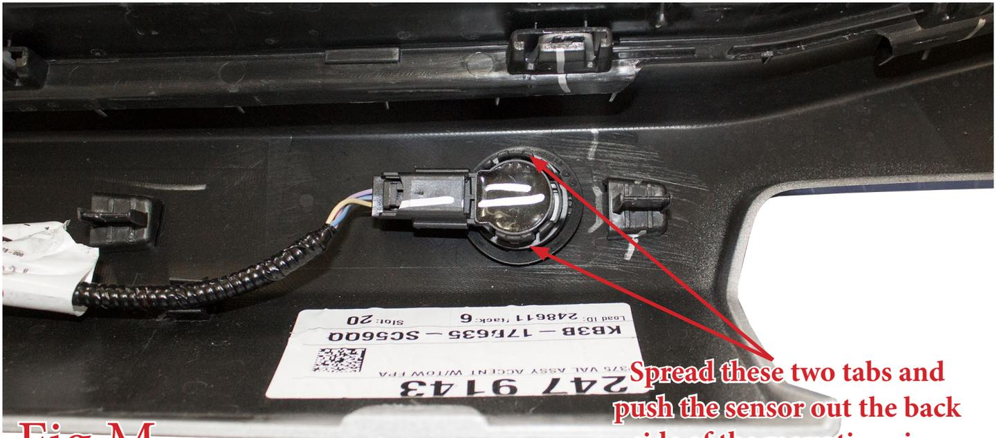
**Spread these two tabs and push the sensor out the back side of the mounting ring**
