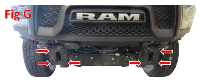
Secure the bumper to the truck using the supplied 1/2" Bolts (x6), 1/2" Washers (x12), and 1/2" Lock Nuts (x6). Leave these bolts finger tight for now. If you are keeping your tow hooks on the truck, use the bottom two bumper mounting bolts on each side to hold the hooks in place. (Fig H)
