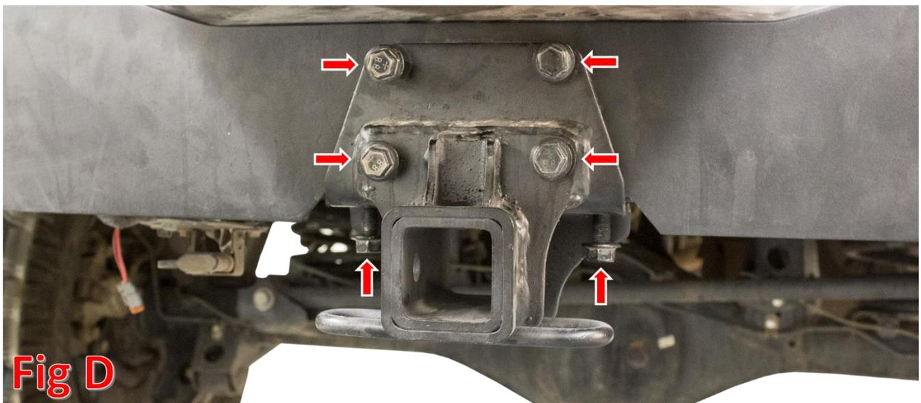
7. Align the bumper so it sits straight in relation to the rear fender body line and is centered left to right. Then, go back and torque the mounting bolts to the manufacturer's torque specifications.
