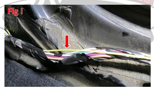
13. Using the splice connector that is already attached to the red LED Harness wire, attach the red harness wire to the Jeep's yellow/white stripe wire. Fig J explains how the splice connector works.
