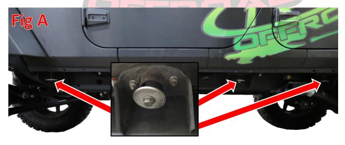
2. Hold your new Side Steps in place, then reinstall the mounting bolts. For the front two mounts, use the supplied M12 Bolts with the OEM Jeep Washers. For the rear mount, use the OEM Bolt/Washer combination. (Fig B) On the front mount, install one of the supplied spacers between the Jeep body and the Side Step Mount (Fig C). Leave these bolts loose for now.
