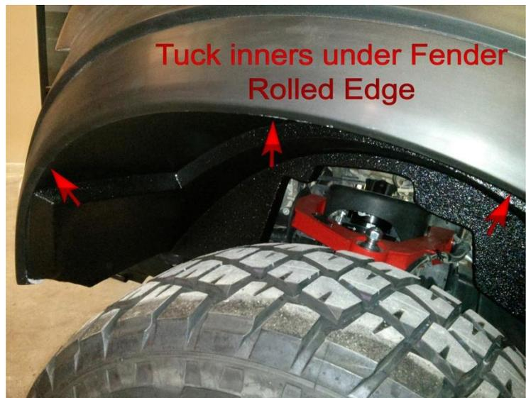
8. Now that fit is verified, remove the Fender Inners and have the inside covered with bedliner material (i.e. Line-x, rhinoliner or equivalent).
