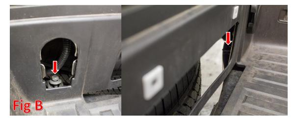
4. Remove the two 18mm Rear Bed Bolts. They are along the rear of the frame, where it meets the hitch tube. Refer to Fig C. Save these bolts for reuse.
