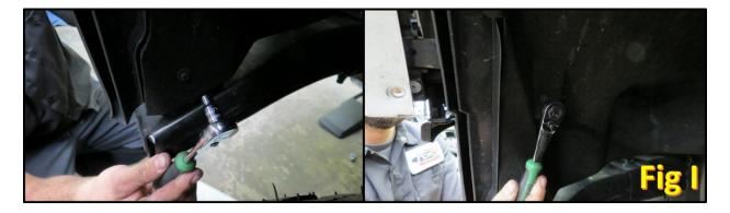
12. Remove the 3 bolts referenced in Fig J on the air dam that sits behind the headlight bezel.
