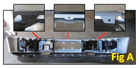
3. Carefully remove the front plastic piece from the bumper. There are no tools required for this, it can be pulled off by hand.
