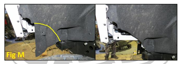
17. Remove the two plastic clips that hold on the rubber piece shown in Fig M. The clip locations are referenced in Fig N.
