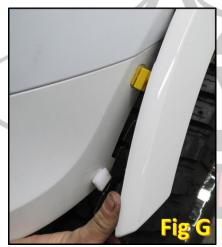
10. Gently pull the headlight bezel forward and off of the vehicle. Refer to Fig H
