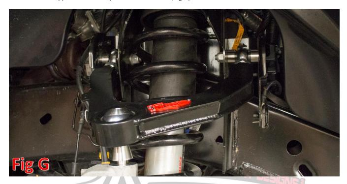
3. Use the OEM Bolts you removed in Removal Step 6 to secure the Upper Arms to the vehicle. For an easier installation, we install the bolts from the outside of the shock tower. Leave these bolts loose for now. On the passenger side of the vehicle, you will have to loosen the ABS controller (three 10mm bolts) to be able to fit the front bolt in. (Fig H)
