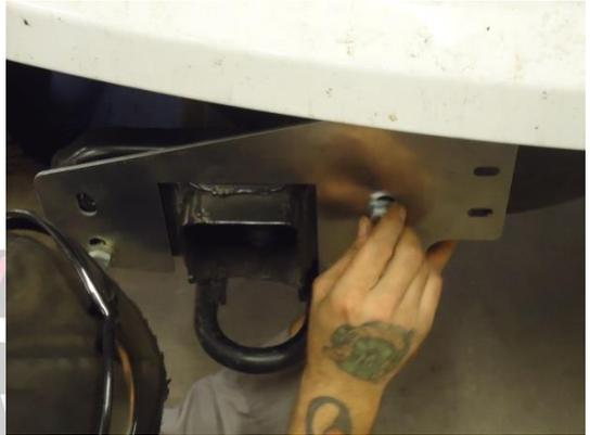
1. Bolt aluminum cooler mount between the two outer aluminum mounts using the provided 6 - 3/8" button head bolts. Tighten these to 20 - 25 ft/lbs. at this time.
