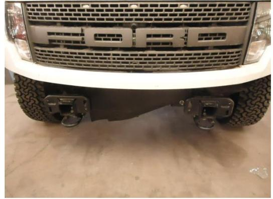
2. Attach the Two(2) aluminum mount plates to the frame horns, using the 2 holes per side that line up. Leave the hardware loose at this point.
