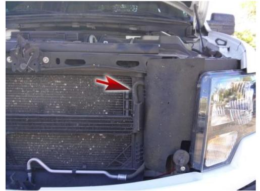
5. Safely route the hoses from the cooler unit to the fittings exposed in step 5 on the factory cooler and the radiator. Cut the hoses to length leaving some play for flex.
