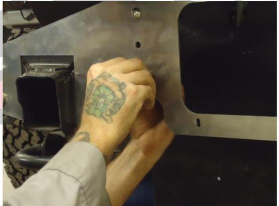
2. Drill the 4 remaining holes, 2 holes on the aluminum mount plates on each side, to 1/2".
