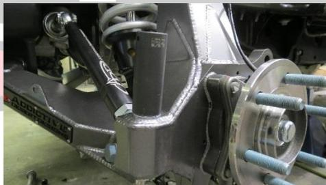
10. Bolt steering clevis to rack using supplied hardware and 3/4 socket. Apply red Loctite to threads. Keep clevis straight up and down. Then bolt tie rod into clevis.
