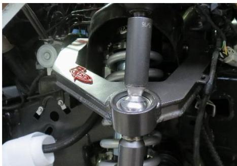
7. Now you will move on to the A-arm mount and frame using a 1" 1/16 socket and wrench.
