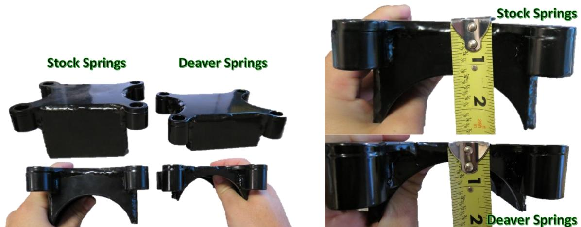
16. Locate the bump stop mount pad assembly and u-bolts. Set the bump stop pad on the top of the axle tube near the spring perch. Slide the u-bolt up from the bottom of the axle assembly through the mounting holes in the bump stop pad assembly. This will fit just between the shock mount and the spring perch on the axle. Make sure the bump stop pad is aligned on the axle to meet the bump stop when the suspension collapses. Follow step 17 for the correct alignment.
