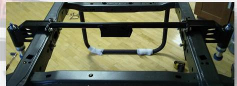
9. Locate the 1/2" x 1/2" Grade 8 Bolts with washers to secure the triangular frame support to the cross member through the 2 holes. Make sure you put washers on the bolts on both sides and install the nut on the threaded end. Tighten these bolts now.
