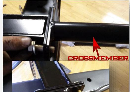
7. Install 4 of the 1/2" x 1/2" Grade 8 Bolts with washers through the cross member outer mounting plate to attach it to the bump stop mount assembly. Use washers and start the nuts. \*\*\*\*Do not tighten bolts yet.
