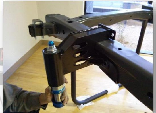
14. Tighten the top nut on both bump stops to ensure they are secure. Replace the Schrader valve cap.
