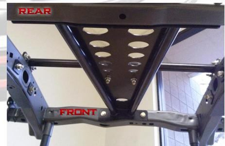
10. Next, locate the 2 holes in the front smaller side of the triangular frame support. Take the 90' drill and 1/2" drill bit and drill through the frame assembly through both sides of the cross member. Install 4 1/2" x 1/2" Grade 8 Bolts to secure the triangular frame support to the factory cross member. Make sure you use washers and put the nuts on the threaded end of the bolt. \*\*\*\*Do not tighten the bolts yet.
