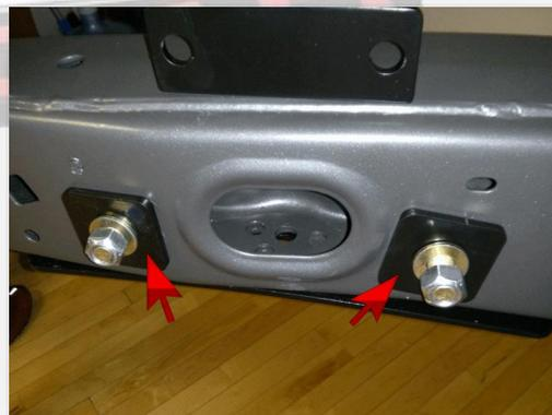
6. Locate the 1-1/2" tube cross member. Slide the tube up over the exhaust and on top of the frame rail. Line these plates up with the bump stop can assembly.
