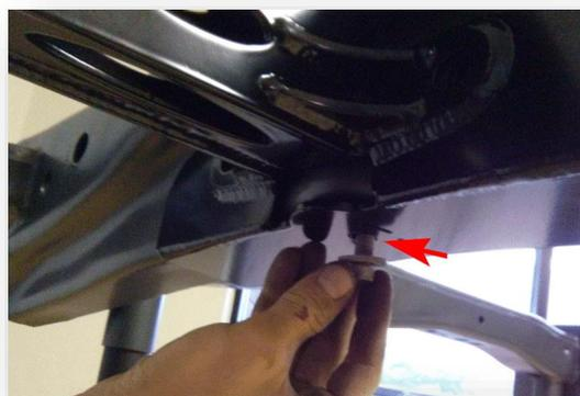
3. Using the Bump Stop Assemblies as a template, drill a 1/2" hole through the frame gusset and into the inside portion of the stock frame. Pay attention to drill as straight as possible.
